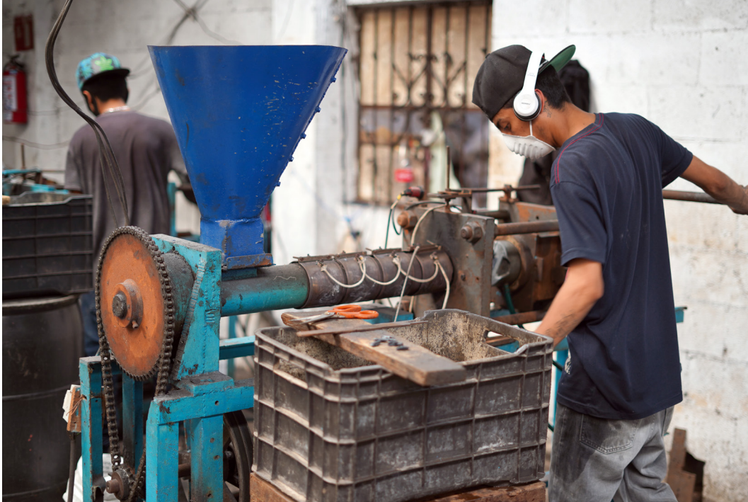
Workers carrying out the process of compaction of plastic by pressure and heat. Photo: Iván Hernández
