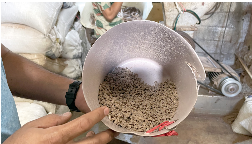
Shredded material from recycled plastic. Photo: Iván Hernández
