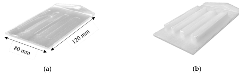
Figure 1. (a) Initial part thickness of 3 mm; (b) the extended ribs height 8.5 mm after cavity expansion.
