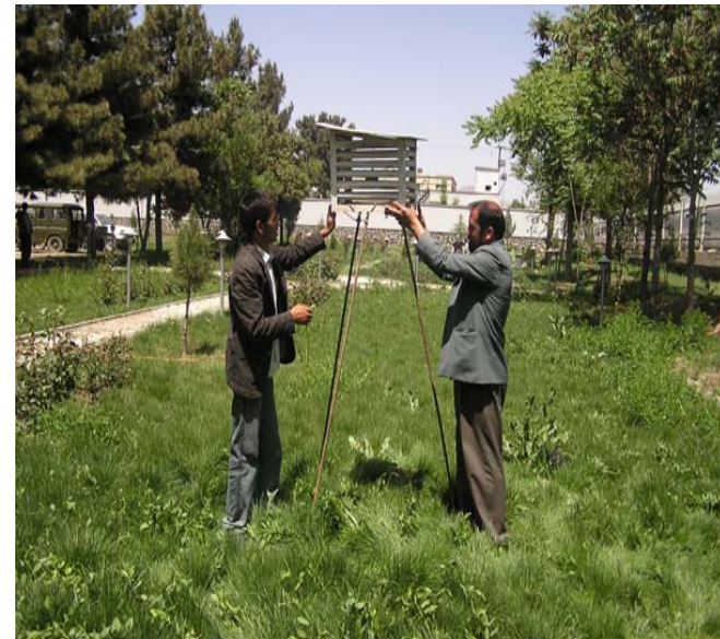
View of HOBO data logger installation in one of the urban gardens in Kabul, Afghanistan.
