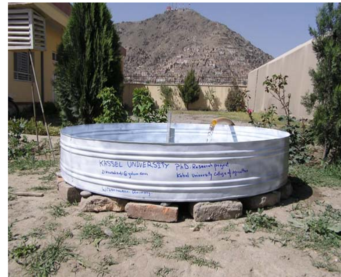
Self-made American Class A-Pan for measurement of potential evaporation in Kabul city, Afghanistan.
