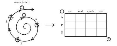
Figure 8. The combination of macro- and micro cycle provides a generic, hypercyclic model of the design process, which can be linearized into a tabular scheme
