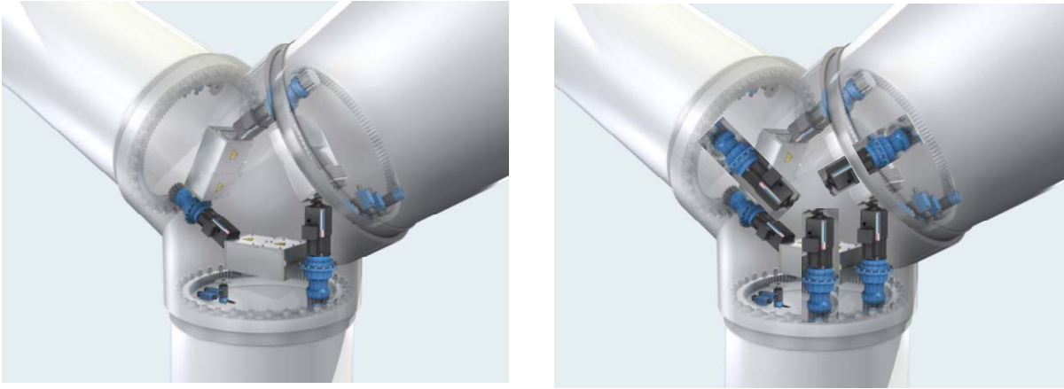
Figure 2-6: current pitch actuation system (left) and the suggested pitch actuation system (right)
