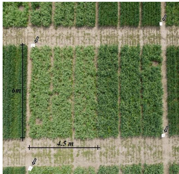
Fig.7.1: Aerial photograph of experimental plots at 60 days after sowing (DAS). Arrows indicate the ground control points, plot size ( 4.5 \times 6 m).
