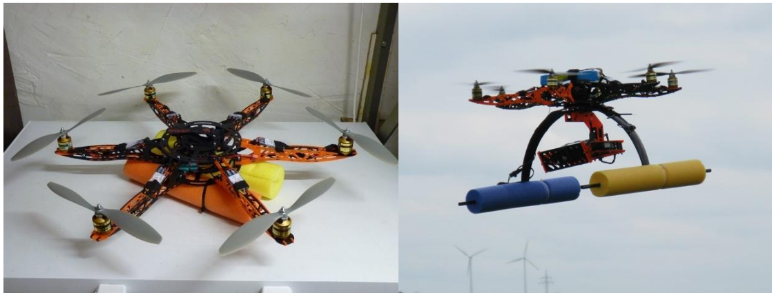
Fig.7. 3: Hexacopter used to take low-altitude aerial photographs.
