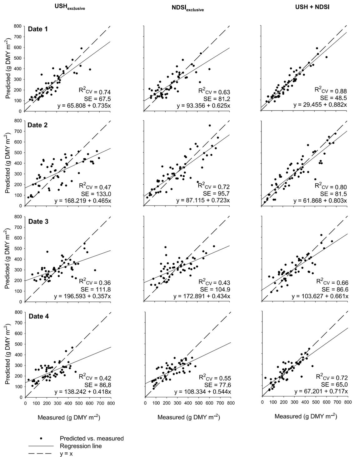
**Figure 4.** Plots of fit between measured and predicted dry matter yield (DMY) for exclusive use of ultrasonic sward height (USH<sub>exclusive</sub>) and the best fit normalized difference spectral index (NDSI<sub>exclusive</sub>) as well as a combination of USH and NDSI (USH + NDSI) applied in date-specific swards.
