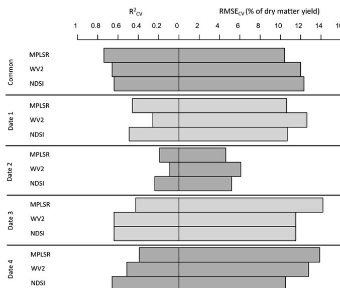
**Figure 3.** Cross-validation (CV) results for a range of sensor models used for prediction of dead material proportion (DMP), including exclusive use of all hyperspectral wavebands using modified partial least squares regression (MPLSR), normalized difference spectral index (NDSI), and multispectral representation of WorldView-2 wavebands (WV2) as explanatory variables.
