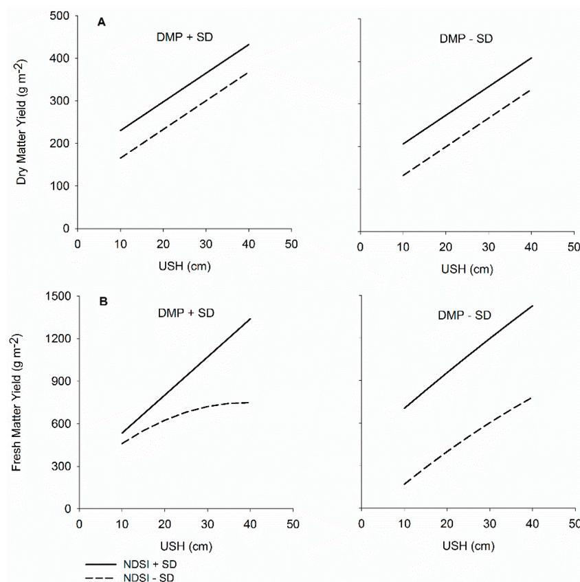
**Figure 5.** Predictions of dry matter yield (DMY) (A); and fresh matter yield (FMY) (B) in common swards based on ultrasonic sward height (USH) and the Normalized Difference Spectral Index (NDSI) as influenced by dead material proportion (DMP) in the range of  $\pm$  standard deviation (SD). NDSI represents narrow-band reflection values selected in combination with USH for each parameter.
