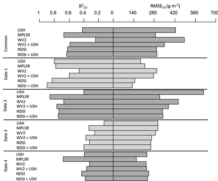
**Figure 2.** Cross-validation (CV) results for a range of sensor models used for prediction of dry matter yield (DMY), including exclusive use of ultra-sonic sward height (USH), all hyperspectral wavebands using modified partial least squares regression (MPLSR), normalized difference spectral index (NDSI), and multispectral representation of WorldView-2 wavebands (WV2), as well as models formed from combinations of these sensors.
