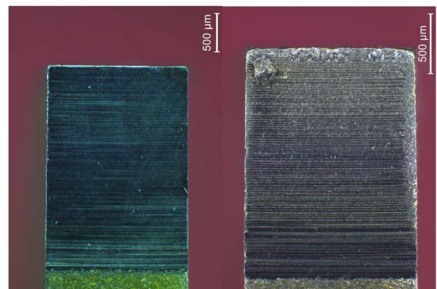
(b) Flank face implanted tool before (left) and after (right) 1200 m length of cut
