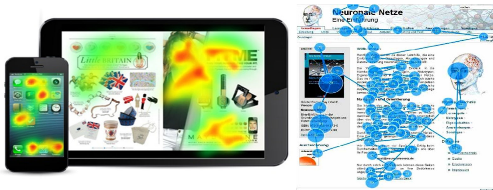
Fig. 2 -Exemplary illustration of a heat map on the left and a Gaze plots right (Strandvall 2017; Rey, 2015)
