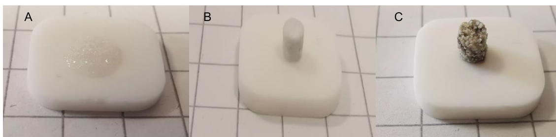
Figure 22: Ash samples after testing the ash melting behavior until the measuring range of 1,500 °C is reached: (A) Untreated wheat straw (B) SW30_a140B (C) SCW30_a140B.
