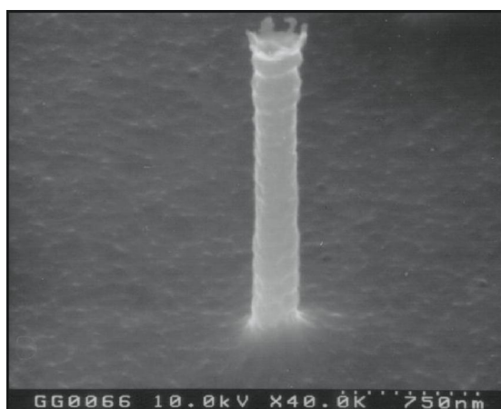
Figure 5.2. a) SEM image of monolayer of 500 nm glass spheres on silicon substrate; b) Top view of the resulting surface structure after applying gas chopping plasma etching reveals silicon pillars of hexagonal cross section; c) Zoom image of b) showing a single 20 nm silicon bridge that connects adjacent pillars; d) Tilted view of the pillars.
