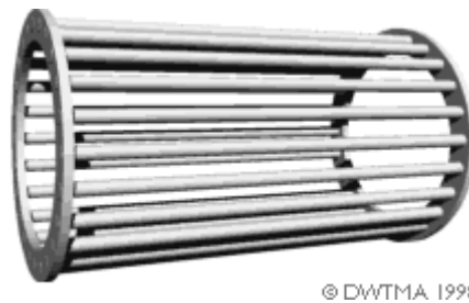
Fig. 4.29: The simplified view of squirrel cage rotor
