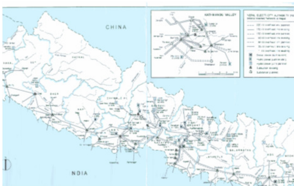
Fig. 3.3: 132 kV transmission, 800 km long running parallel to Indian border, connects big cities across the country [4]
