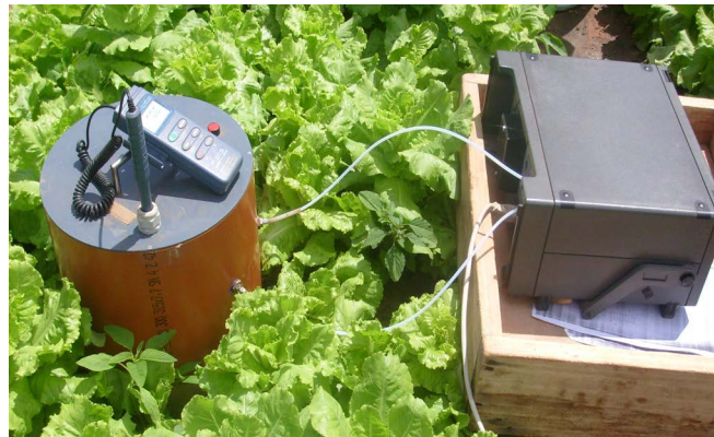
Picture 3. A closed chamber system consisting of a cuvette connected to a photo-acoustic infrared gas analyzer INNOVA 1312-5
