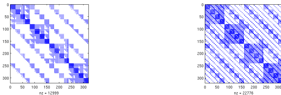
Figure 5.2: Sparsity pattern of a diagonal (left) and offdiagonal (right) for the Navier-Stokes equations.
