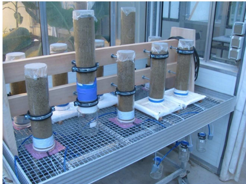
Fig. 2. Picture of the experimental design. Treatments from left to right: Glass suction plate, ion exchange resin cartridge, glass suction plate, two PE suction plates. PE = Polyethylene.
