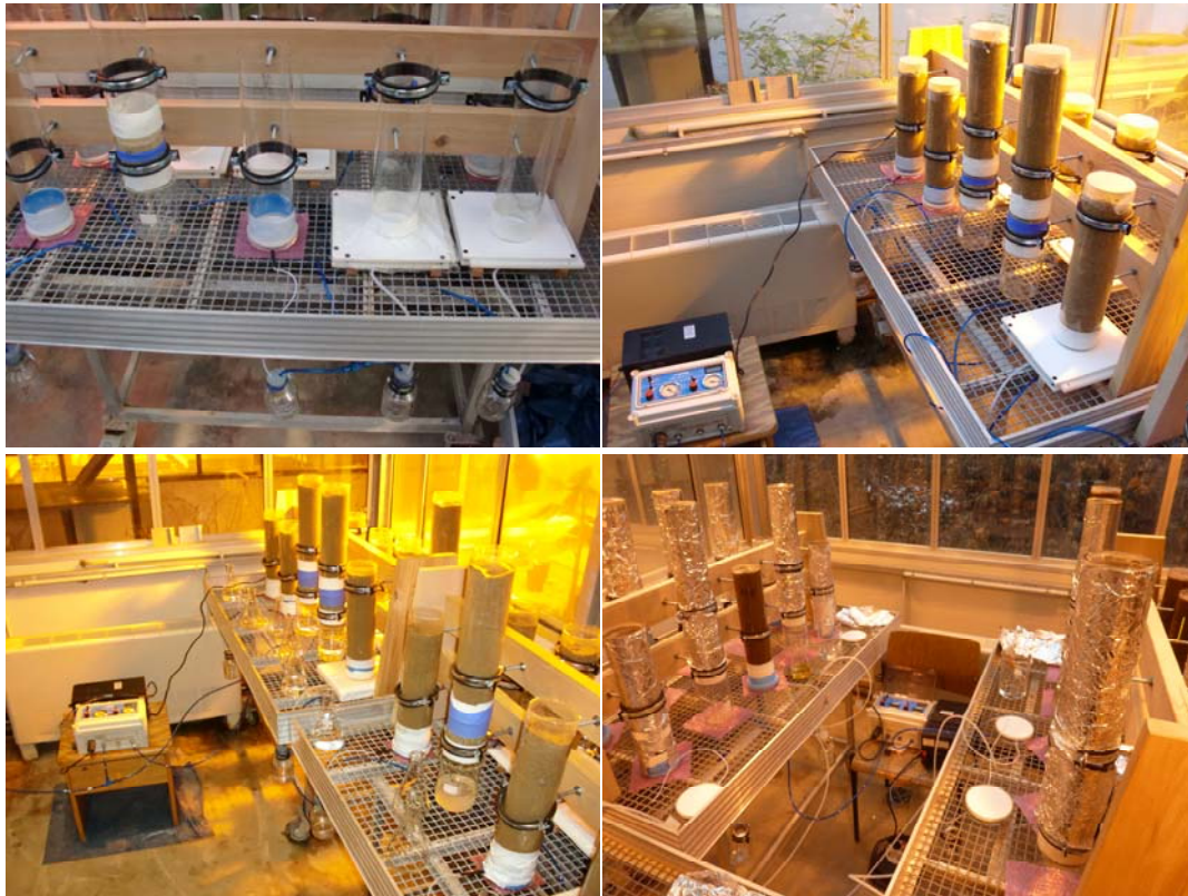
Fig. 2. Pictures of the experimental setup. Upper left and upper right pictures: Glass cylinders are attached to glass suction plates, glass resin boxes (= resin cartridges), or PE suction plates (from left to right). Suction plates are connected to sampling bottles via PTFE tubes. Lower left picture: Sampling bottles are connected to a vacuum pump, whereas percolate from resin cartridges drains freely into glass collection beaker. Lower right picture: Soil columns are covered with aluminum foil to avoid algae growth.
