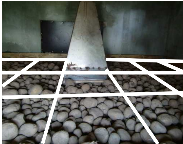
Figure 7-3 pictorial view of tapered channel used for measuring bulk potatoes headspace air velocities.
