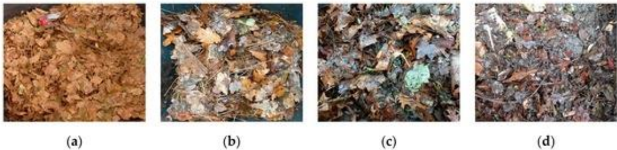
Figure 3.1 Exemplary display of leaf litter material immediately after collection by two different techniques: the vacuum technique in (a) residential areas during a dry period and (b) on main roads during a wet period; and the sweeping technique in (c) residential areas and (d) in city centres, both during a wet period.
